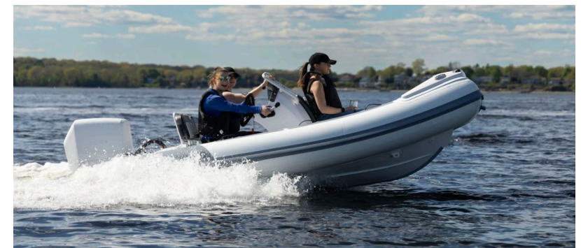
Flux Marine, rigid inflatable with battery electric outboard motor
