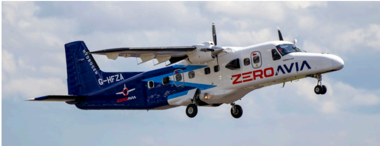
ZeroAvia Successfully Completes Initial Dornier 228 Flight Test Campaign with prototype ZA600 hydrogen-electric engine [Kemble, UK & Hollister, CA: 19th July, 2023] zeroavia.com
