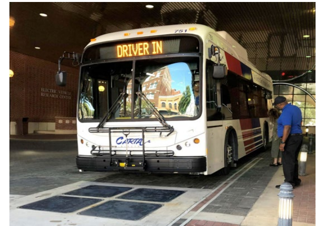
Example of inductive charging capabilities (Source: CARTA)
